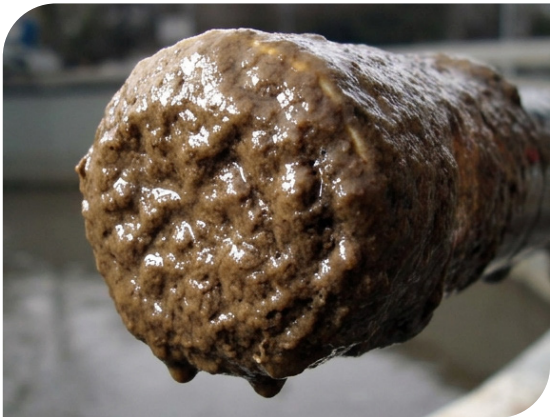
VisoTurb sensor without UltraClean ultrasonic cleaning activated, after a 30-day deployment.
