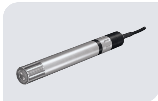
The VisoTurb uses a nephelometric measurement principle and integrated UltraClean ultrasonic cleaning for continuous turbidity and TSS monitoring.
