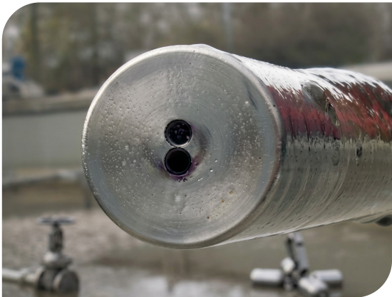
VisoTurb sensor with UltraClean ultrasonic cleaning activated, after a 30-day deployment.
